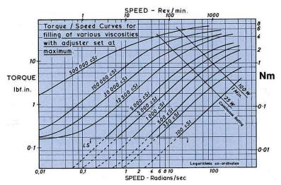
The S-CRD continuous rotation dashpot has an adjustable rate. Specification of a given silicone fluid filling provides maximum rates as shown by the curves opposite.
